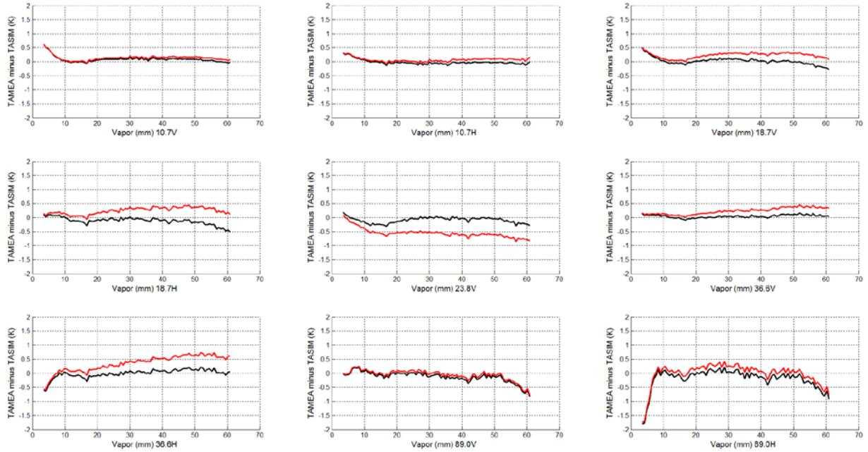
**Figure 4.** Differences between measured and RTM computed antenna temperatures for the 9 lowest GMI channels. The black curves show the results for the absorption model in this paper (same as in Figure 1). The red curves show the results if the air-broadened half-width for the 22 GHz vapor line is decreased by 5% as suggested in *Liljegren et al.* [2005].
