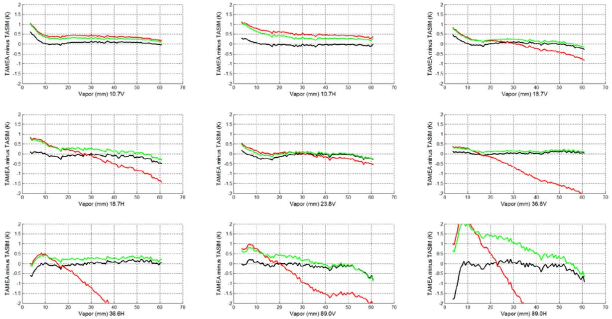
**Figure 1.** Measured minus RTM computed antenna temperatures for the 9 lowest GMI channels: Red curves: using the dry air coefficients given by *Liebe* [1989] and *Liebe et al.* [1992] and the vapor coefficients given by *Rosenkranz* [1998]. Green curves: after adjusting the water vapor absorption. Black curves: after adjusting both water vapor and dry air absorption.
