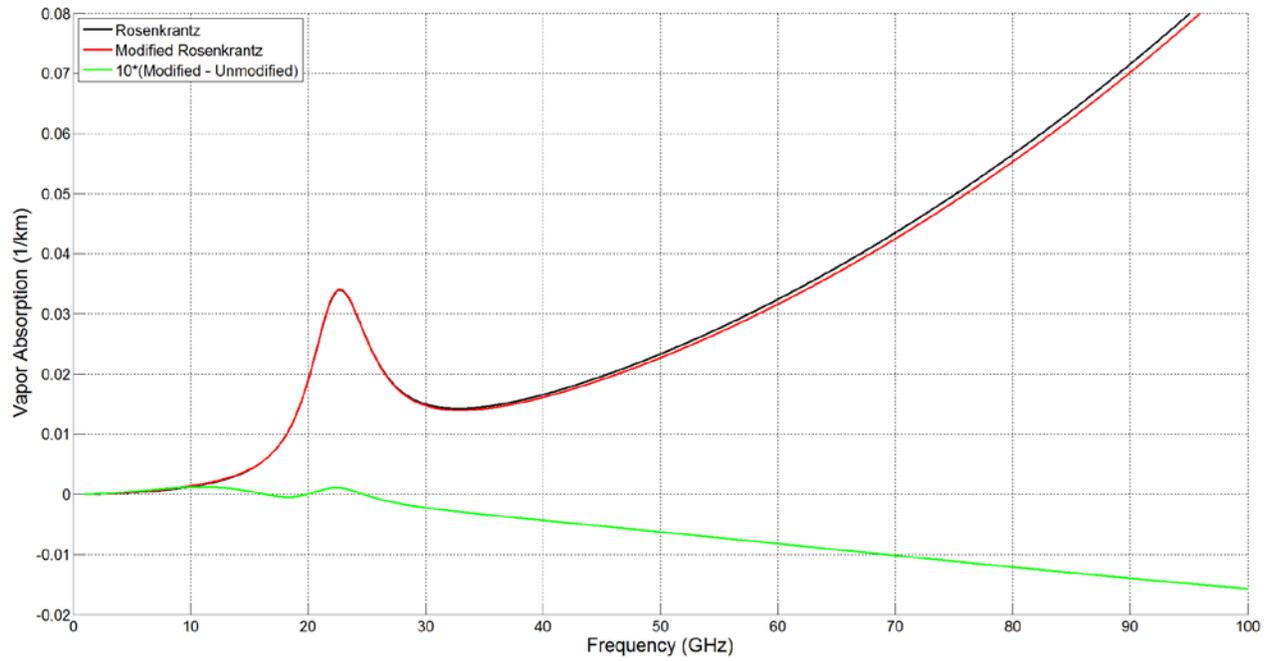
**Figure 2.** Total water vapor absorption ( $\text{km}^{-1}$ ) from *Rosenkrantz* [1998] (black curve) and after making the adjustments in this paper (red curve). The green curve shows 10-times the difference between the adjusted and unadjusted water vapor absorption model.
