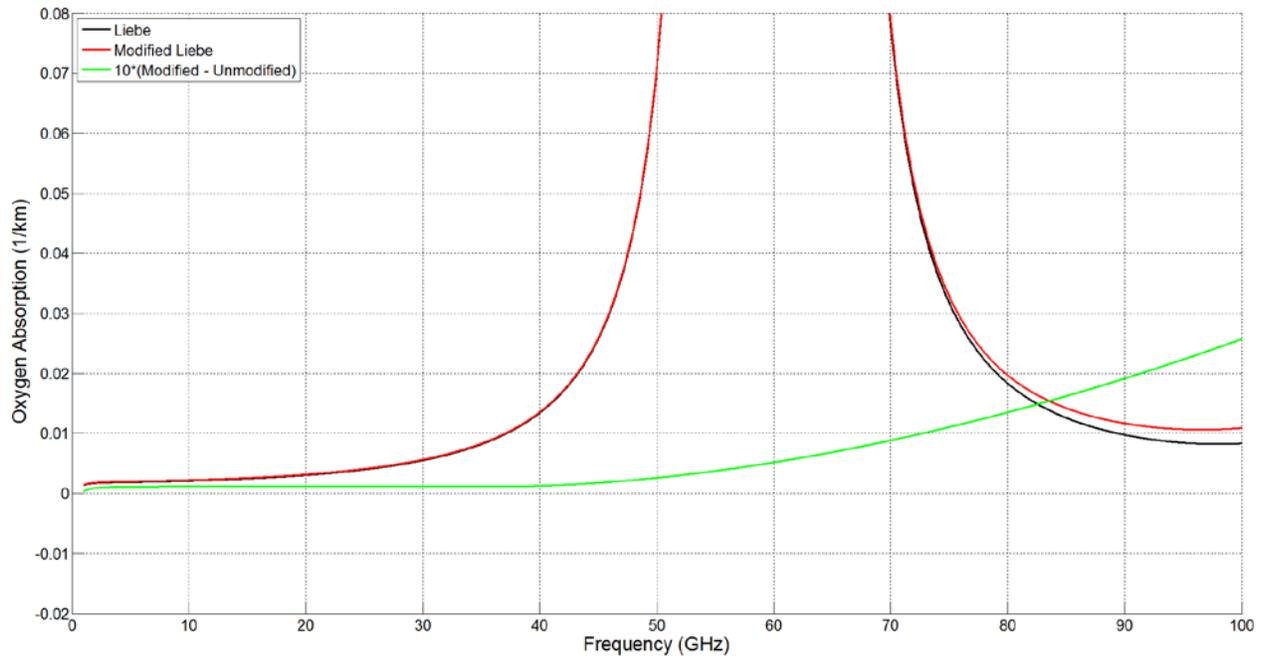
**Figure 3.** Total dry air absorption ( $\text{km}^{-1}$ ) from *Liebe et al.* [1992] (black curve) and after making the adjustments in this paper (red curve). The green curve shows 10-times the difference between the adjusted and unadjusted dry air absorption model.
