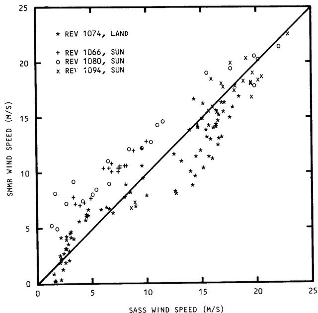
Fig. 6. A scatter plot of SMMR versus SASS winds for four North Atlantic revs. affected by land and sun glitter. The line of perfect agreement is shown.
