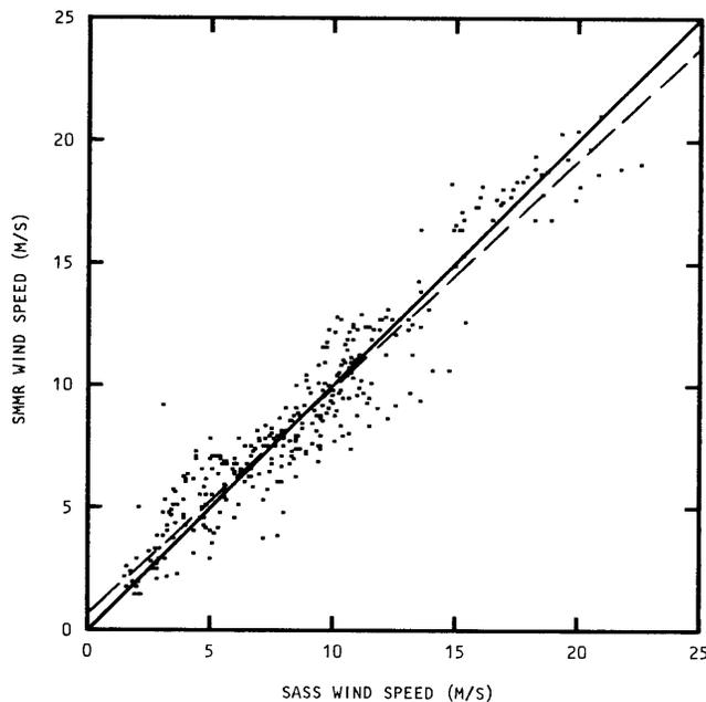
Fig. 5. A scatter plot of SMMR versus SASS winds for six North Pacific revs. Line of perfect agreement is the solid line, and the least squares fit is the dashed line.
