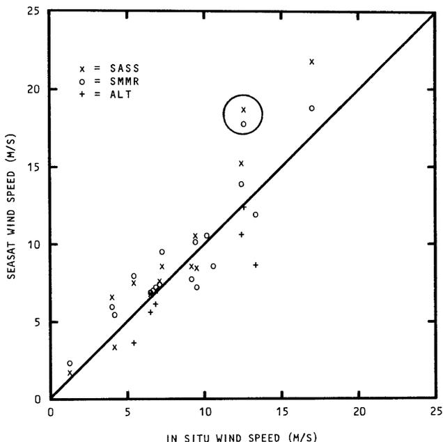
Fig. 3. SASS, ALT, and SMMR inferred wind speeds plotted versus in situ anemometer observations. The line of perfect agreement is shown.
