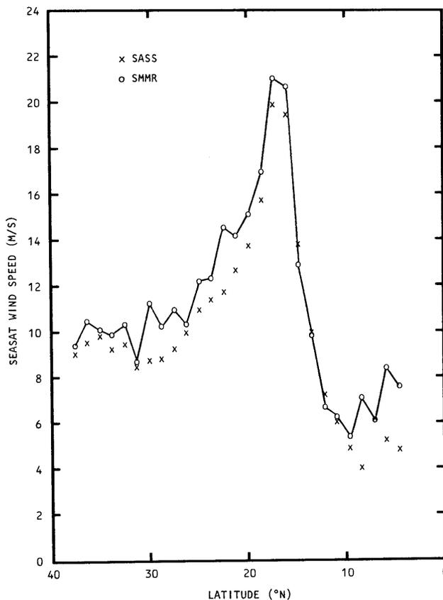
Fig. 7. A comparison of SASS and SMMR wind speeds for Hurricane Fico for grid 1, column 3 of rev. 331.
