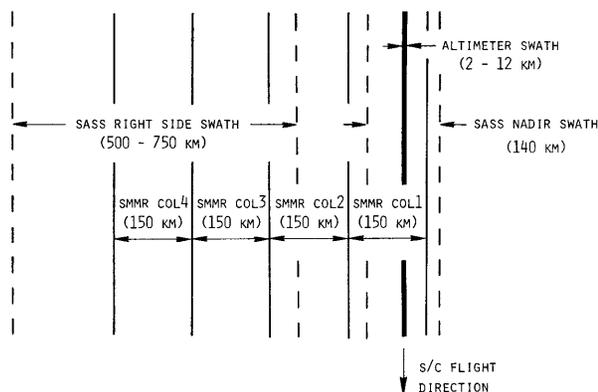
Fig. 1. Rightside swath coverage for the SASS, ALT, and SMMR.
