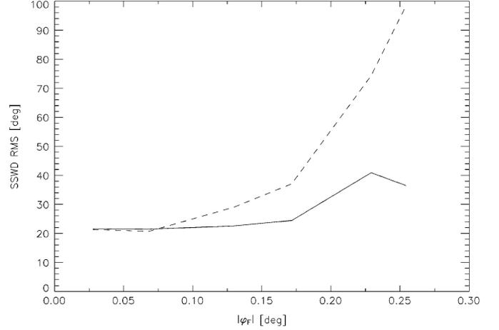
Fig. 6. RMS difference between the wind direction of the NCEP GDAS analysis and the closest ambiguity of the wind vector retrieved from WindSat for wind speeds larger than 5 m/s plotted as a function of the absolute value of the Faraday rotation angle. The computation was done for 30 orbits (rev # 3720–3749). The bin size is  $0.025^\circ$ . The full (dashed) line shows the result if the Faraday rotation was included (not included) in the cross-polarization correction.
