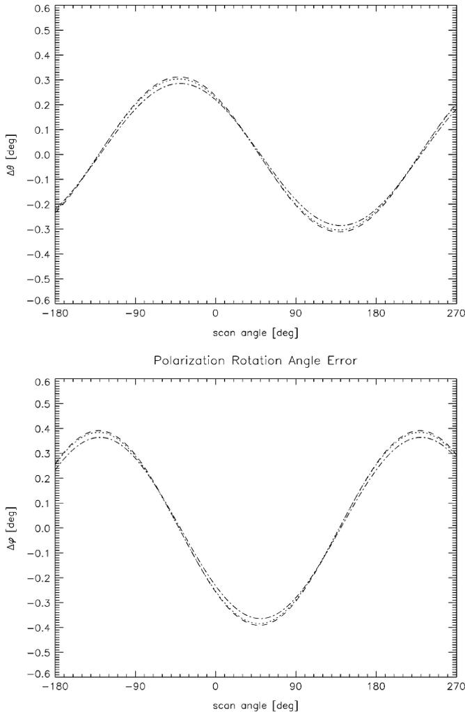
Fig. 3. Error in the EIA  $\Delta\theta$  and the polarization rotation angle  $\Delta\varphi$  for the orbits from Fig. 2 as function of the antenna boresight looking azimuth (scan angle) at (dotted line) 10.7, (dashed line) 18.7, and (dashed-dotted line) 37.0 GHz.
