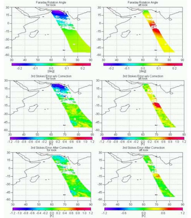
Fig. 5. Faraday rotation at 10.7 GHz and error in the 10.7-GHz third Stokes parameter (measurement minus RTM function) for orbit rev # 3733 (September 26, 2003). The left (right) panels show forward (aft) look. The upper panels show the magnitude and size of the Faraday rotation angle. The middle (lower) panels show the error in the third Stokes parameter without (with) including Faraday rotation in the polarization rotation correction.
