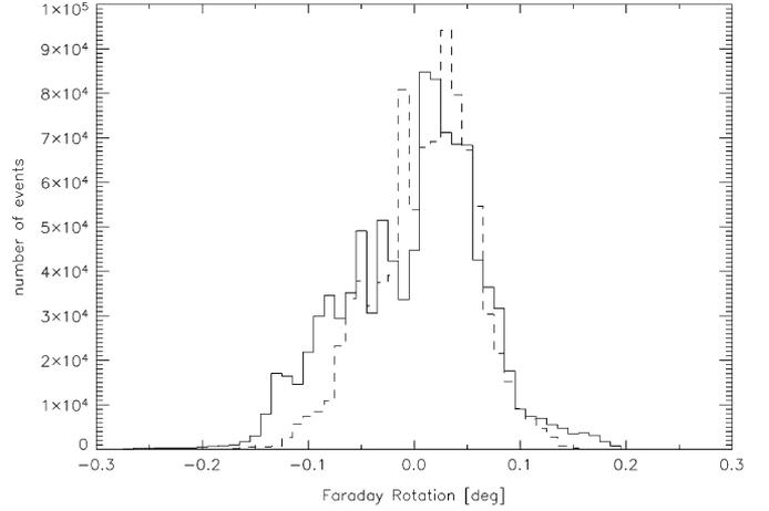
Fig. 4. Distribution of Faraday Rotation angles over the ocean for two 30-orbit periods. (Full line) Rev # 3720–rev # 3749 (September 25–27, 2003) and (dashed line) rev # 5211–rev # 5240 (January 8–10, 2004). The bin size is  $0.01^\circ$ . The observations were averaged into target cells matching the size of the 10.7-GHz footprint.
