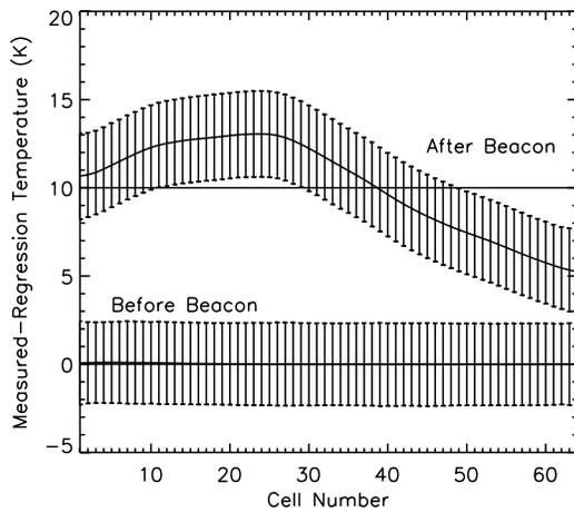
**Figure 1.** Cell position average difference between the measured and the regression-predicted 22 GHz vertical-polarization brightness temperature before the beacon was turned on (year 2005) and after (year 2007). These averages are for the rain-free ocean equatorward of 60 degrees latitude for the 64 SSM/I footprints along the scan. The “after” curve is our correction.
