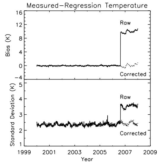
**Figure 2.** Daily-average time series of the difference between the measured and regression-predicted 22 GHz vertical-polarization brightness temperature for raw F15 data (solid curve) and the corrected F15 data (dotted curve). The (top) bias and (bottom) standard deviation are shown, and the calculations are over the rain-free global-ocean equatorward of 60 degrees latitude.
