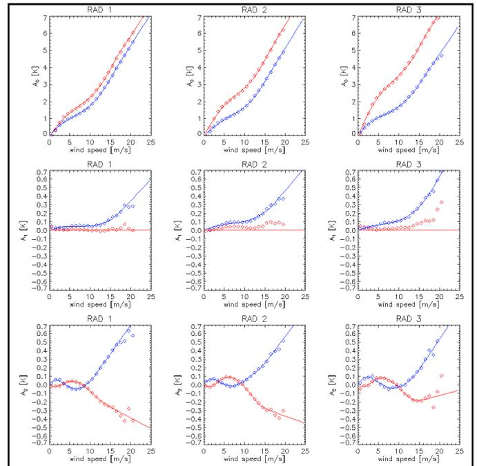
Figure 1: Harmonic coefficients of the expansion (1) of the wind induced surface brightness temperature  $\Delta E_w \cdot T_s$  (in Kelvin) for the 3 Aquarius radiometers: blue = v-pol, red=h-pol. The Earth incidence angles for the beams are: 28.7° (RAD 1), 37.9° (RAD 2) and 45.5° (RAD 3).
