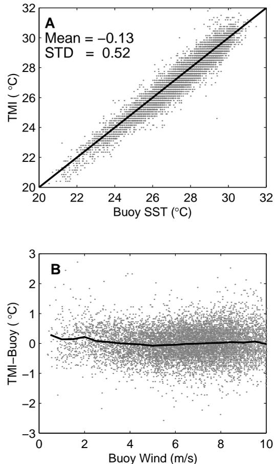
Fig. 1. TMI SST comparisons to TAO/TRITON Buoy SST. 1998 and 1999 data were collocated to within one hour and 0.5°. A) TMI SST versus Buoy SSTs. B) TMI - Buoy SSTs versus Buoy wind speeds.
