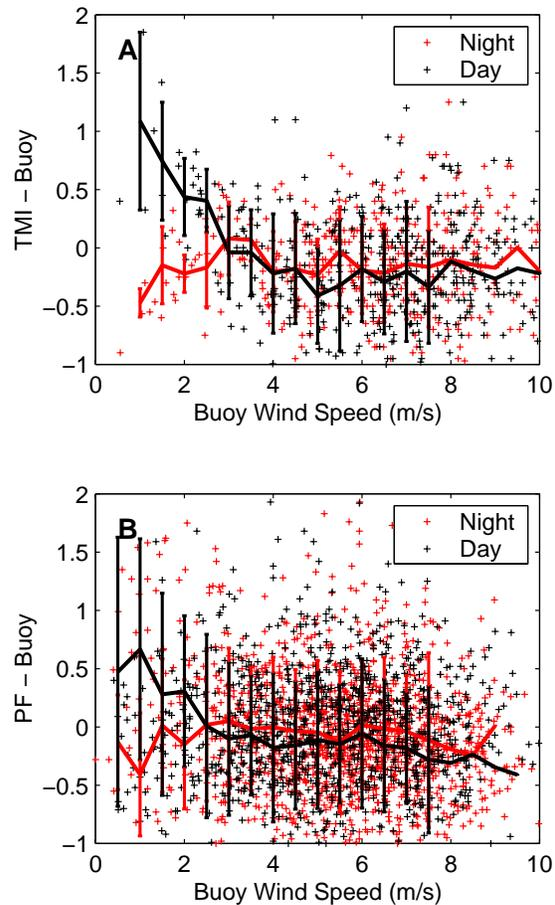
Fig. 3. Diurnal skin effects from satellite SSTs. A) TMI - Buoy SST versus Buoy Wind Speed. B) Pathfinder - Buoy SST versus Buoy Wind Speed. In both figures, black is used for daytime data and red for nighttime data. Pathfinder has an equatorial crossing time of 2:30.
