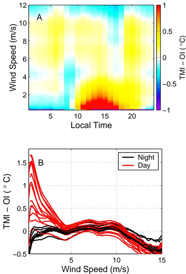
Fig. 4. Diurnal skin effects from TMI and OI SSTs. A) Image of the average difference, TMI - OI as a function of local time and wind speed. B) Average difference, TMI - OI SST, for each local time hour, versus wind speed. Nighttime data is presented in black, daytime in red.
