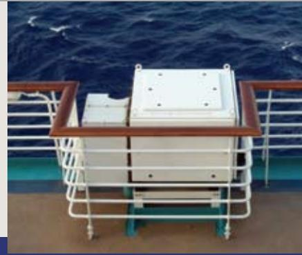
The Marine-Atmospheric Emitted Radiance Interferometer (M-AERI), which accurately measures the ocean's skin temperature.
