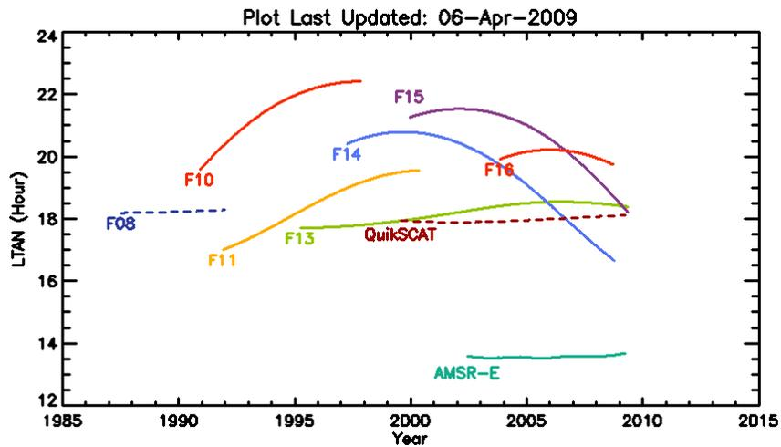
**Figure 2.** Time series of local equatorial crossing time. Dashed curves indicate that descending time is plotted. F15 is the purple curve.
