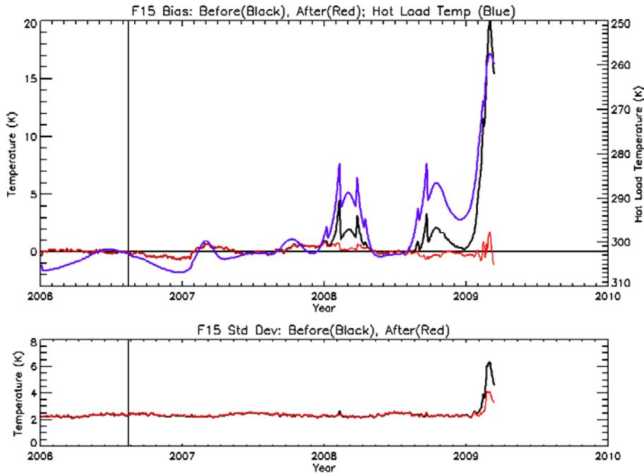
**Figure 4.** Time series of the measured minus predicted 22V brightness temperature bias (top) and standard deviation (bottom). Shown are: data corrected with HW08 (black line), data corrected with the temperature dependent correction in this report (red line), and the hot load temperature (blue line, which corresponds to the right axis). Note: the right axis for hot load temperature is reversed.
