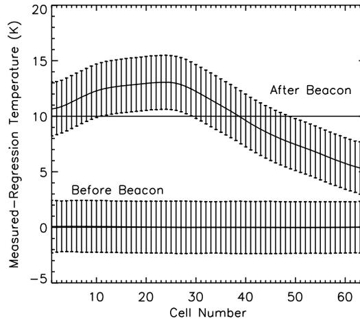
**Figure 1.** Cell-average difference between the measured and predicted 22V brightness temperature before the beacon was turned on (year 2005) and after (year 2007). These averages are for the rain-free ocean equatorward of 60 degrees latitude for the 64 SSM/I footprints along the scan. The “after” curve is the HW08 correction.
