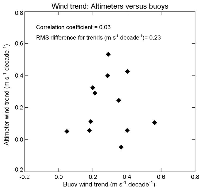
**Fig. 1.** Plot of altimeter versus buoy wind trends ( $\text{m s}^{-1} \text{ decade}^{-1}$ ) for the 12 selected buoys, as given in table 1 of Young *et al.* (5). The figure includes the correlation coefficient and the RMS difference for buoy minus altimeter wind trends. For a mean global wind of  $7.5 \text{ m/s}$ , the RMS corresponds to  $3.1\% \text{ decade}^{-1}$ .
