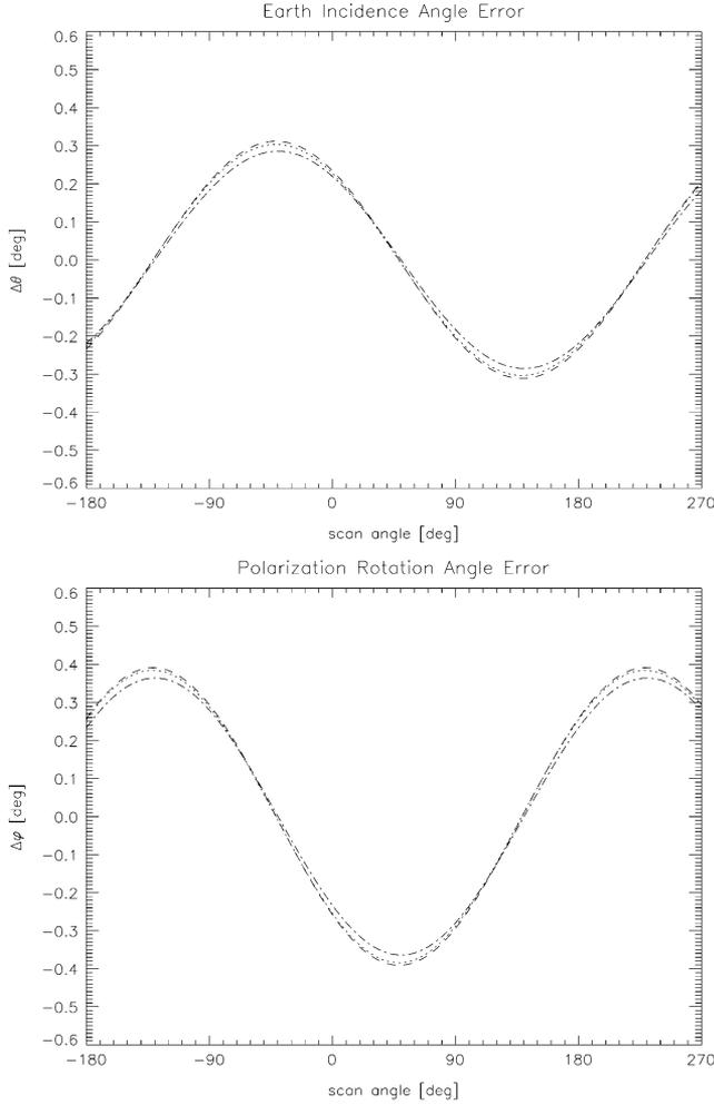
Fig. 6. Error in the EIA  $\theta$  and the polarization rotation angle  $\varphi$  as function of the antenna boresight looking azimuth (scan angle) at (dotted line) 10.7, (dashed line) 18.7, and (dashed-dotted line) 37.0 GHz.
