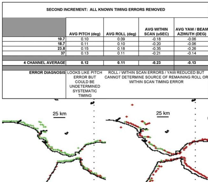
Fig. 4. Geolocation performance in second increment. The table summarizes the average error for several datasets taken from various geographic locations with various pass geometries. The images show a close-up image of local maxima in an area slightly smaller than  $3^\circ$  latitude  $\times$   $3^\circ$  longitude. The green dots in the local maxima plots represent cross-scan local maxima, while the red dots indicate along-scan local maxima. (Left) Forward scan. (Right) Aft scan.
