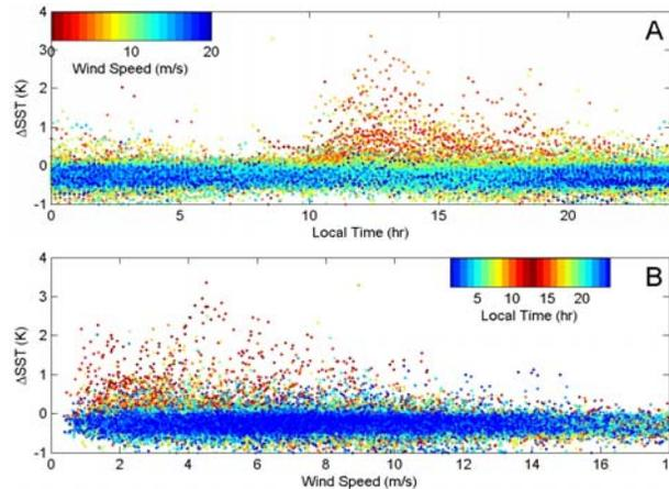
Figure 2. Diurnal warming as a function of local time and wind speed. The difference, skin minus bulk SST is shown 2A, with wind speed indicated by dot color and in 2B as a function of wind speed with local time indicated by dot color.
