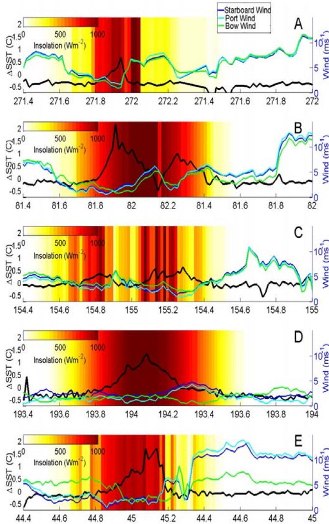
Figure 3. Several examples of diurnal warming from the *Explorer of the Seas*. The difference, skin minus bulk, is shown on the left axis in black, the wind speed is shown on the right axis in blue, cyan, and green, the insolation is indicated by color in the background, and day of the year is indicated. Panel A is from 2001, panels B-D are from 2002, and panel E is from 2003.
