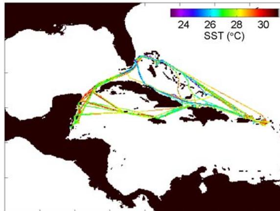
Figure 1. SST along cruise tracks for the *Explorer of the Seas*. Data taken when the ship is in port are not usable, and the diurnal warming analyzed here are from the two days each week that the ship travels to and from Miami on the longer legs. The measured temperature is indicated by color.
