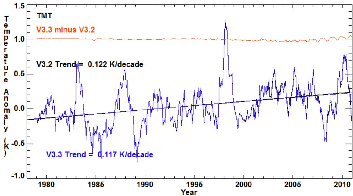
Fig. 7. Tropical (25S to 25N) time series, 1979-2010. Note that despite the reduction in overall trend, by the end of the current time period, V3.3 is warmer than 3.2. This suggests that the trends would become closer together as time goes on, if we chose to continue processing the data using V3.2 methods.
