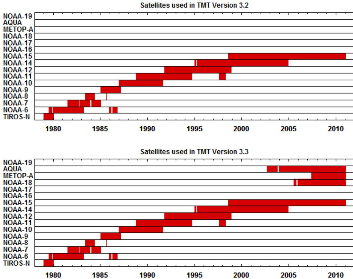
Fig. 1. Time series plots of the satellites used in versions 3.2 and 3.3. Red means that a given satellite is used in the merged product, and white means that it is not used or not present. These plots are for the middle tropospheric channel. Other channels are similar.
