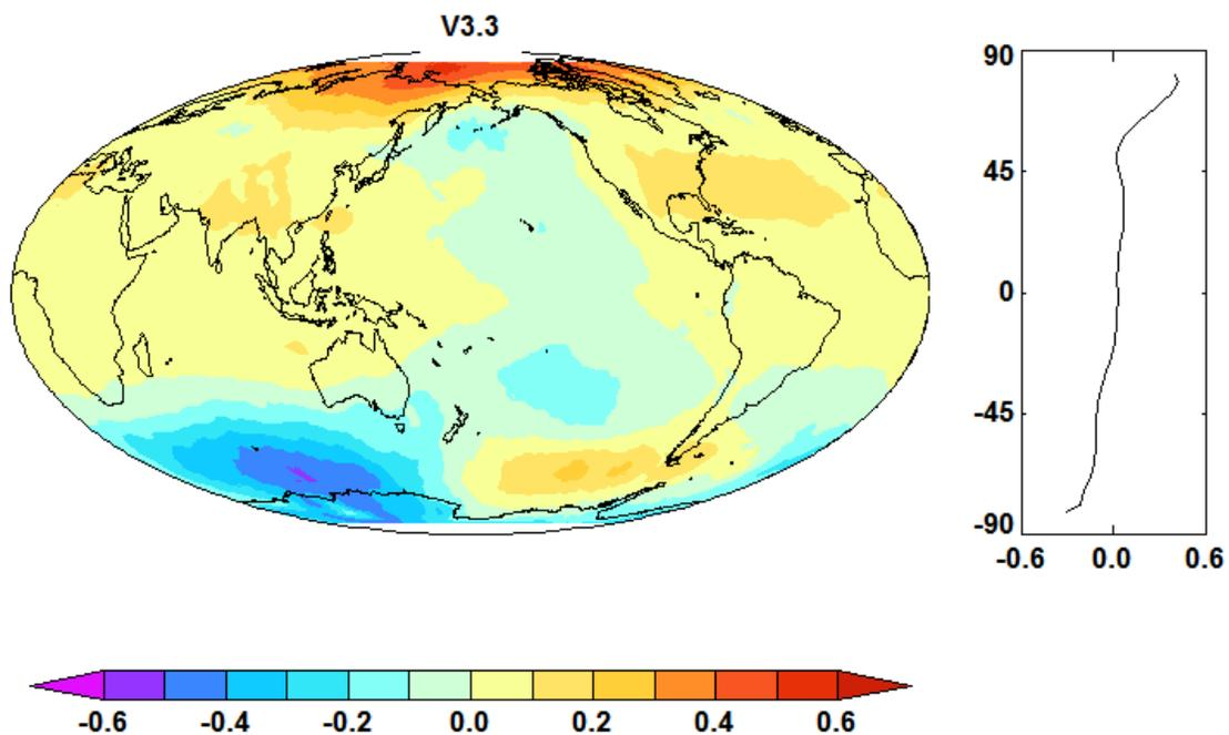
Fig 13. V3.3 TTS Trends. Note reduction in "orbital striping", most visible in the southern ocean. This is due to a reduction in sampling noise for time periods where more AMSUs are available.
